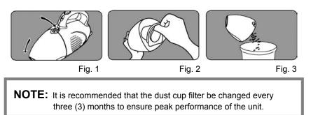
**CAUTION:** The suction hole must be free of obstructions at all times. Otherwise, the motor will overheat and could become damaged.
